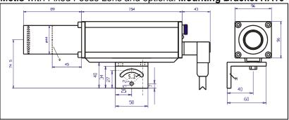
Water Cooling Jacket KG10 and Air Purge BL12 for use of Metis MY in hot ambient up to 200°C
