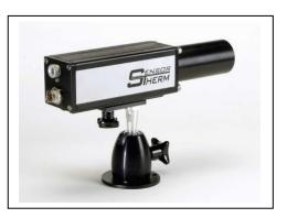
**Optics:** The infrared radiation emanating from the measuring object is transmitted to the detector either via a fixed or focusable optics (MY47 only fixed optics, focused at 600 mm). The lens material used for the optics consists of  $CaF_2$  (calcium fluoride). For measurements through viewing windows, a material with comparable transmission properties should be used.
