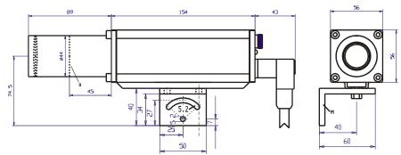
Depending on model, the lens tube length is either 45 mm or 89 mm.
