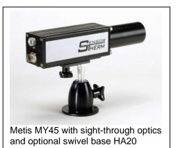
**Optics:** The pyrometer is sensitive to infrared radiation in an area called cone of vision. This area has to be kept free from any intervening objects. The infrared energy radiated by the hot gas is centered via focusable or fixed focus lenses directly on the detector. The focusing feature allows control of the cone of vision and offers the possibility to measure either a small spot (focused) or the average of a bigger spot (out of focus).
