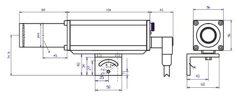
Depending on model, the lens tube length is either 45 mm or 89 mm.
