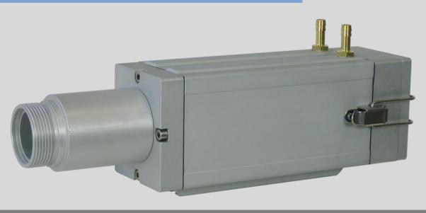
The cooling jacket is used to operate pyrometers outside their permissible ambient temperature up to 250°C. As a cooling medium, water or air can be used, the maximum cooling capacity is achieved only with water. The two quick locks of the back cover allow for quick removal and installation of the pyrometer or the camera. The focusable optics can be adjusted in the cooling housing by unscrewing the optics protection tube from the cooling housing.
